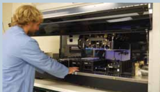
▲ The Hamilton STAR liquid handling system is operated in the A&G drug discovery lab.
